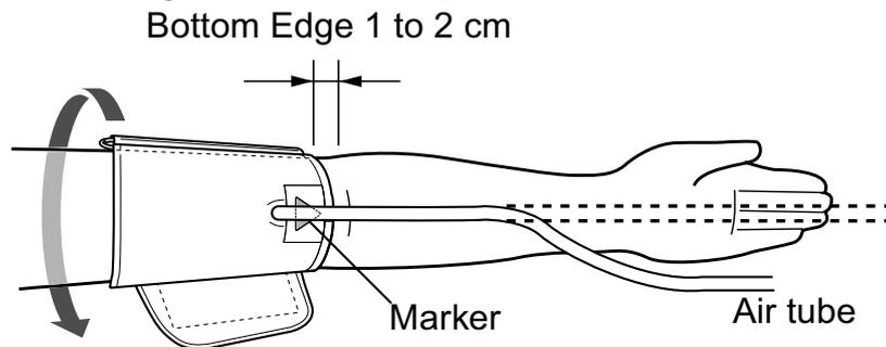
The bottom of the cuff should be approximately 1 to 2 cm above the elbow.
