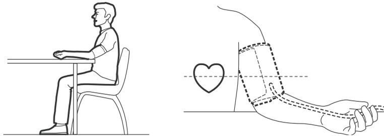
2. Apply the arm cuff to your upper arm. The coloured marker should be centred on the inside of your arm and point down the inside of the arm, so that the air tube runs down the inside of your forearm and is in line with your middle finger.
