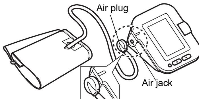
The cuff must be fully deflated when it is inserted into the air jack.
